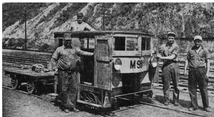
"Section-car de luxe: The Reading and the Jersey Central own several of these, used mainly for Bridge and Building workers who often make long trips in bad weather. Picture was taken at Mauch Chunk, Pa. The boys are proud of their detachable roomette. Note the track-sweeping brooms in front of the wheels"
