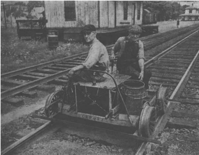
"Lightweight motor-cars, such as this type on the Jersey Central, are designed for two-man welding outfits or other small crews. Observe the safety bar in front of the wheels, to guard against capsizing if the car is derailed"
